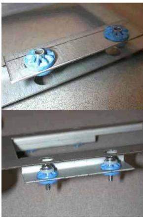
**STEP 3:** Turn the bracket over and insert the (4) 1/2" Long screws thru the white plastic spacers and into the metal standoffs in the blue Grommet.
