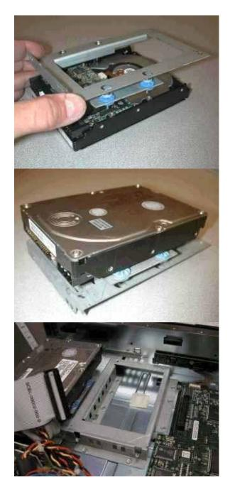
**STEP 7:** Slide the drive bracket into position, lining up the two metal prongs in the TiVo chassis with the holes in the TiVo Mounting Bracket. If you find that the factory-installed bracket is too close to the new bracket that you are now trying to install, you may have to unscrew the factory bracket (which is connected to the factory drive) and move it into the alternate set of holes. Moving the factory bracket over will leave sufficient room for the new bracket.
